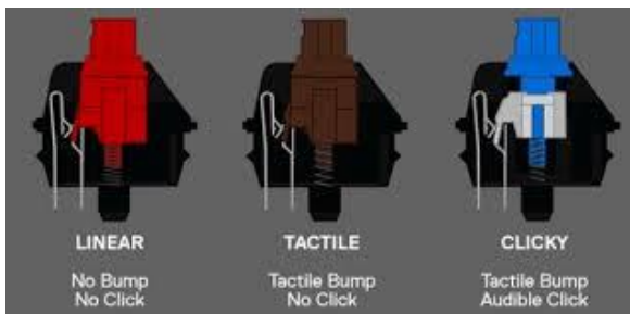
Gambar 2.7 Perbandingan Switch Linear, Tactile, dan Clicky
